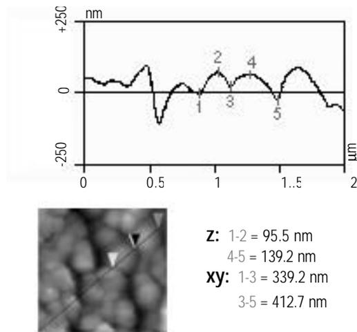
**Figure 2.** AFM section analysis of the nanospheres marked in the image below.
