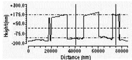
**Figure 4.** Surface profile of a layered sediment of nanospheres.
